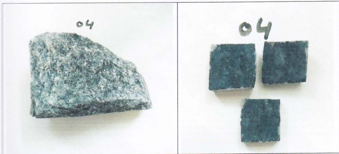
Fig-4.1 Photographs show the supplied rock sample before and after cutting
