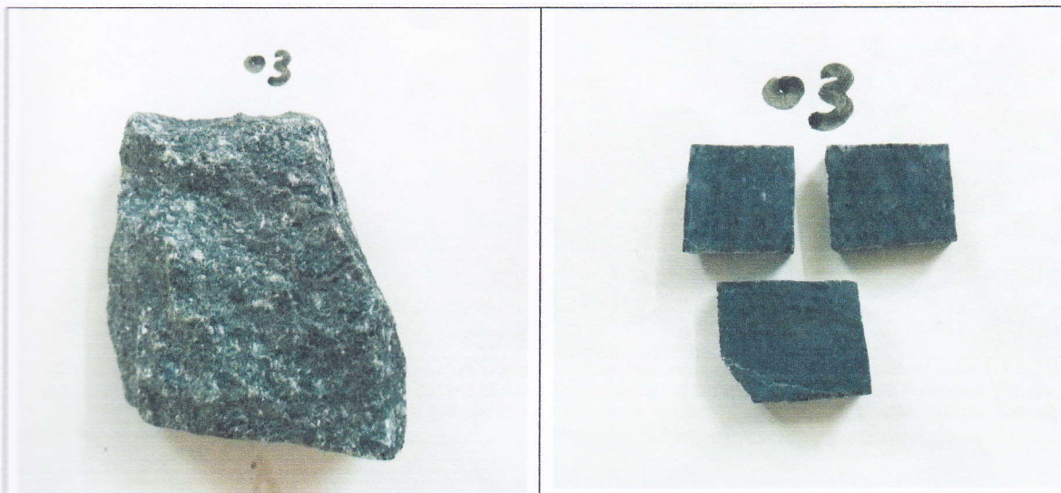
Fig-3.1 Photographs show the supplied rock sample before and after cutting
